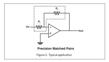
The best analog design would be to use a fundamentally low-absolute-TCR resistor, since it would minimize the effect of ambient temperature and self-heating. This is impossible to accomplish with resistors with high TCR >5 ppm/°C, even with good initial TCR tracking of less than 2 ppm/°C.
