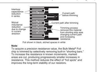
In the fine adjusted areas, trimming affects the final resistance value by smaller and smaller amounts down to 0.001% and finally 0.0005% (5 ppm). This is the trimming resolution (see Figure 4).
