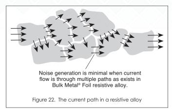
is across the inter-granular boundaries of the alloy. The inter-granular current path from one or more metal crystals to another involves multiple and long current paths through the boundaries, reducing the chance for noise generation. Figure 22 illustrates this current path.
