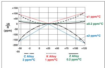
Figure 1. Typical resistance versus temperature curve and its chord slopes (TCR) of foil alloys in military range
