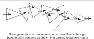
Figure 21. The current path in a particle-to-particle matrix
